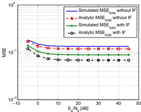
Fig. 7. Comparison between simulated and analytical total MSE performance with 16-QAM constellation and 64-tap channel estimator.
