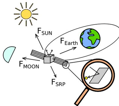
Figure 1: Forces included in the satellite's equation of motion
