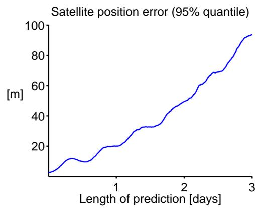
Figure 4: Error in satellite's position as a function of prediction length.
