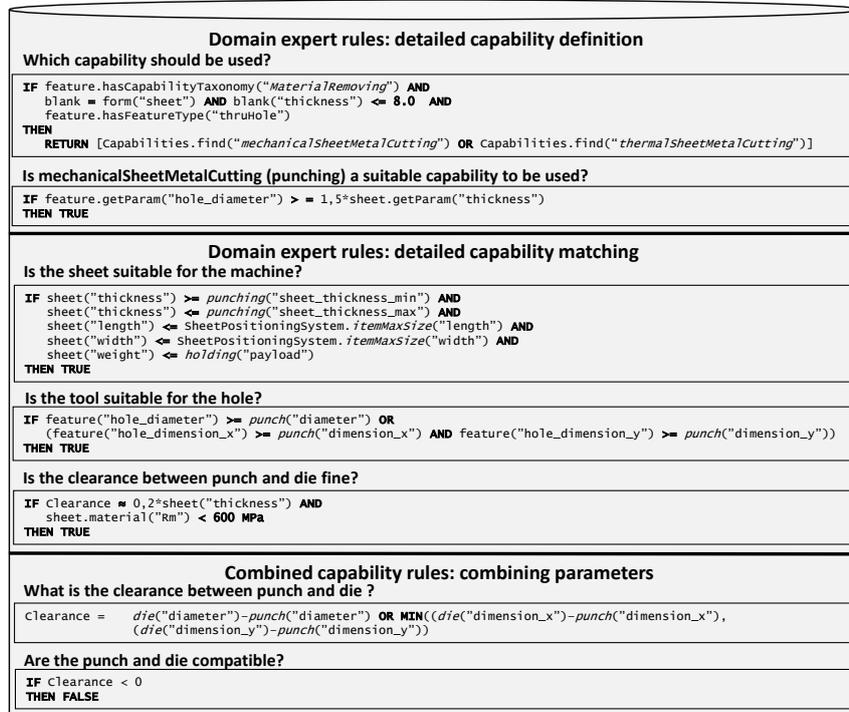
**Fig 1.4** Example of the rules used for capability matching in sheet metal manufacturing written in pseudo code.
