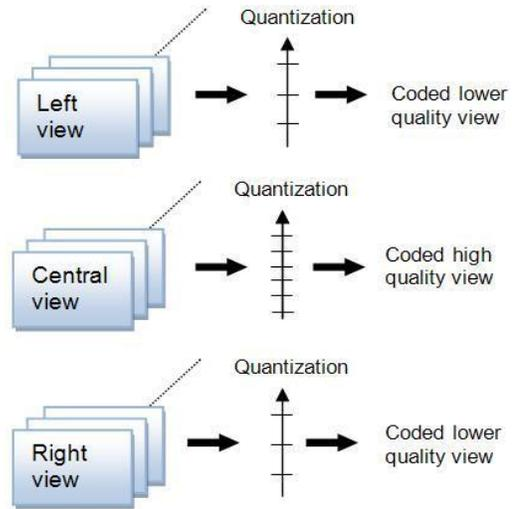
**Fig. 3.** Proposed asymmetric MVC scheme for 3DV coding
