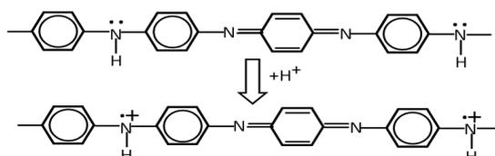
**Figure 2.** Protonic acid doping process of polyaniline.
