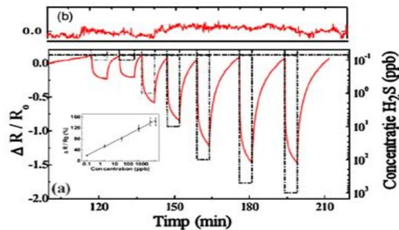
**Figure 5.** Response and recovery transients (solid line) of gold nanoparticles functionalized PANI nanowire network based chemiresistive sensor toward 0.1 ppb, 1 ppb, 10 ppb, 100 ppb, 500 ppb, and 1 ppm (dashed line) concentrations of H<sub>2</sub>S gas.
