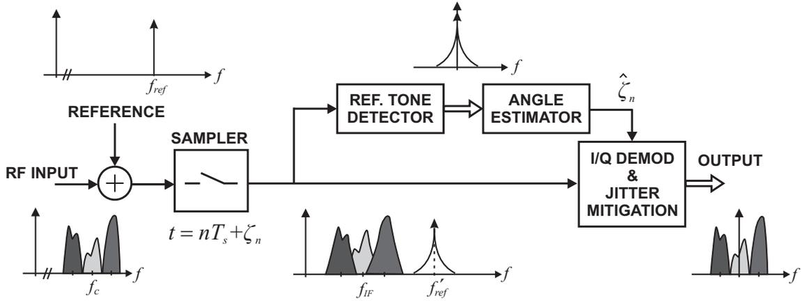
Fig. 1. General illustration of super-imposing a reference tone at sampler input, which is then used for digital jitter estimation and cancellation from the actual received signal in a direct-sampling radio. For illustration purposes, only three received channels are shown, and the target signal is depicted in the lightest grey.
