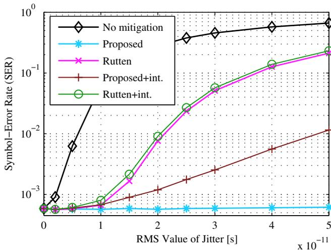
Fig. 4. SER as a function of sampling jitter RMS with fixed SNR of 18 dB in AWGN channel.
