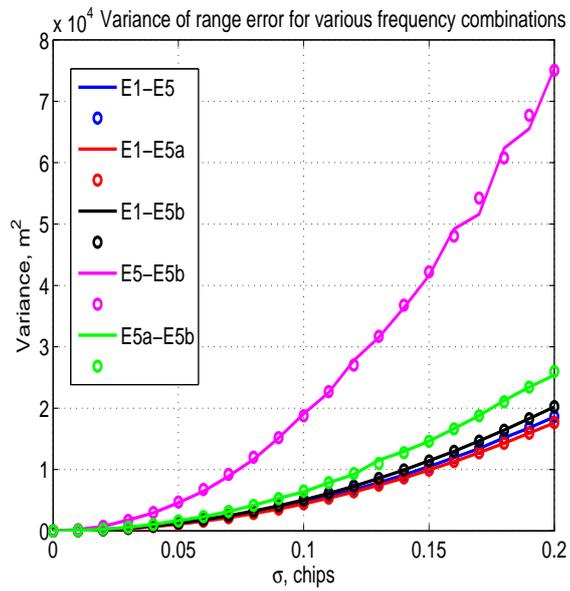
Figure 1: Variance of range error for various frequency combinations and zero mean measurement errors (solid line: simulation-based, filled circle: theory-based)
