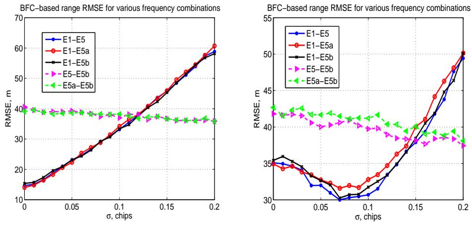
Figure 9: Range RMSE of BFC method for various frequency combinations, zero (left plot) and non-zero mean (right plot).
