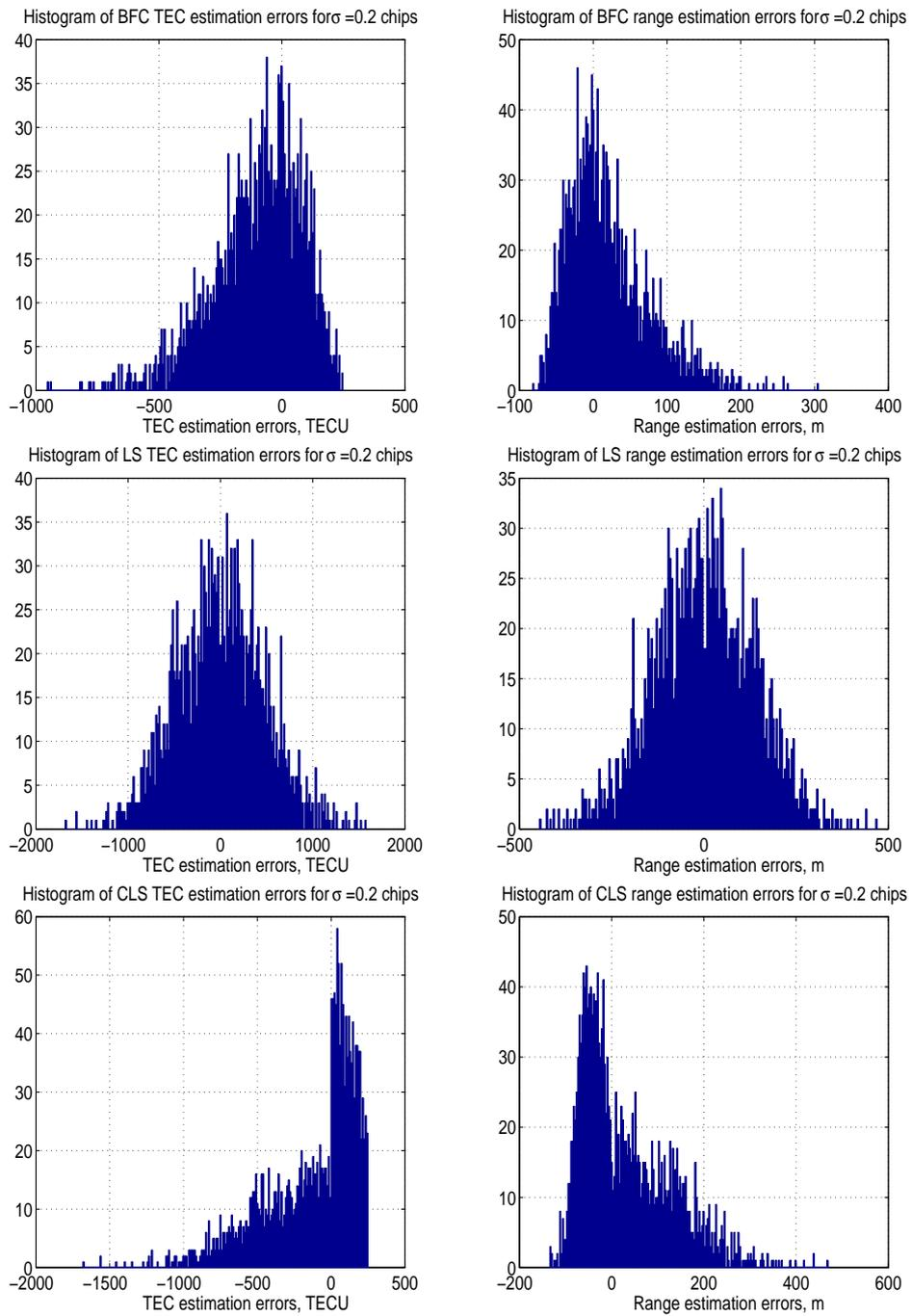
Figure 5: Histograms of TEC and range estimation errors of BFC (top plots), LS (middle plots) and CLS (bottom plots), for E1-E5a frequency combination, zero mean and  $\sigma = 0.2$  chips.
