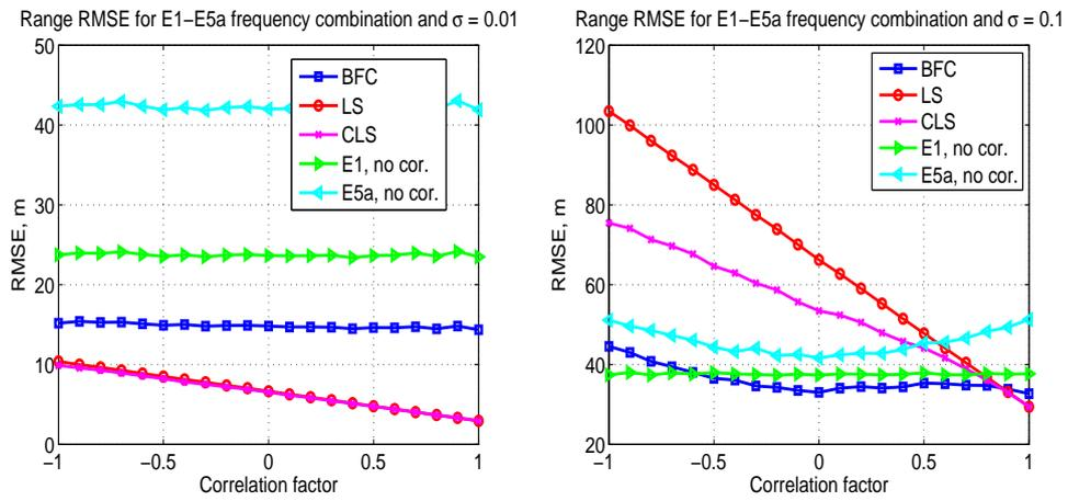
Figure 7: Range RMSE versus correlation factor for E1-E5a frequency combination, zero mean,  $\sigma = 0.01$  (left plot) and  $\sigma = 0.1$  (right plot).
