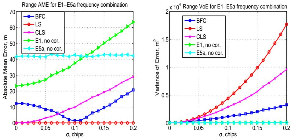
Figure 6: AME (left plot) and VoE (right plot) for E1-E5a frequency combination and zero mean.
