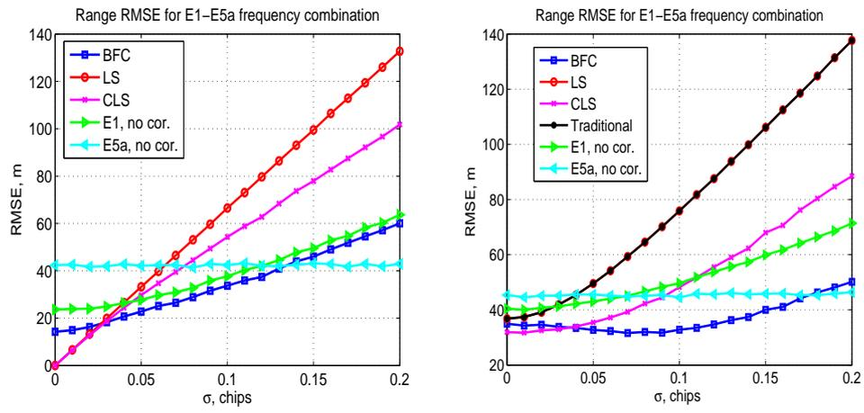
Figure 3: Range RMSE for E1-E5a frequency combination, zero (left plot) and non-zero (right plot) mean.
