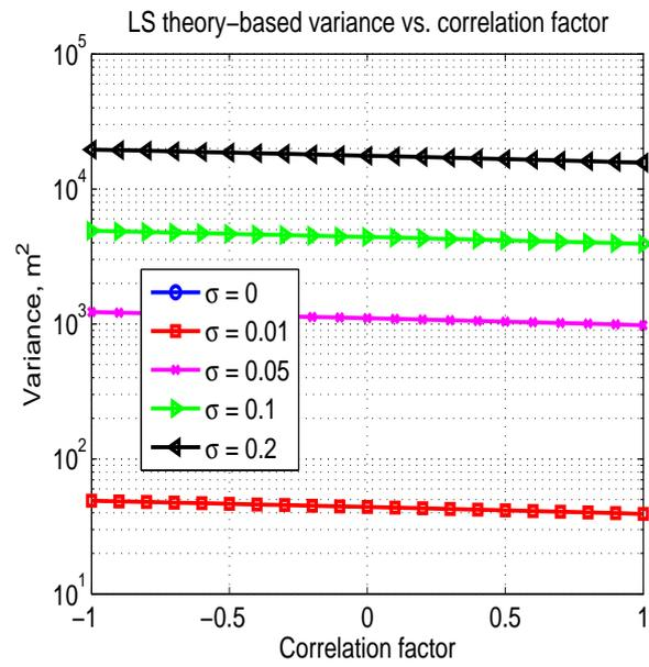
Figure 2: Theory-based variance of LS method versus correlation factor ( $\lambda$ ), for different standard deviations of measurement error ( $\sigma$ ) and mean equal to zero ( $\mu = 0$ ).
