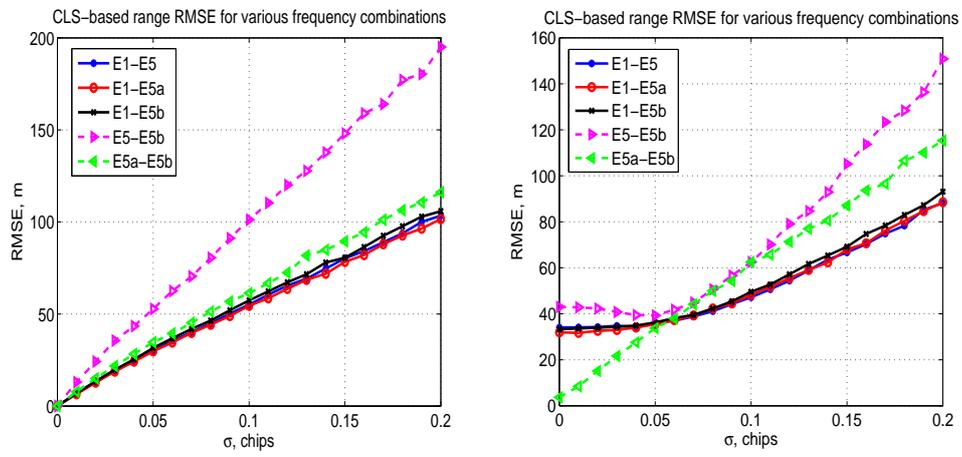
Figure 8: Range RMSE of CLS method for various frequency combinations, zero (left plot) and non-zero mean (right plot).
