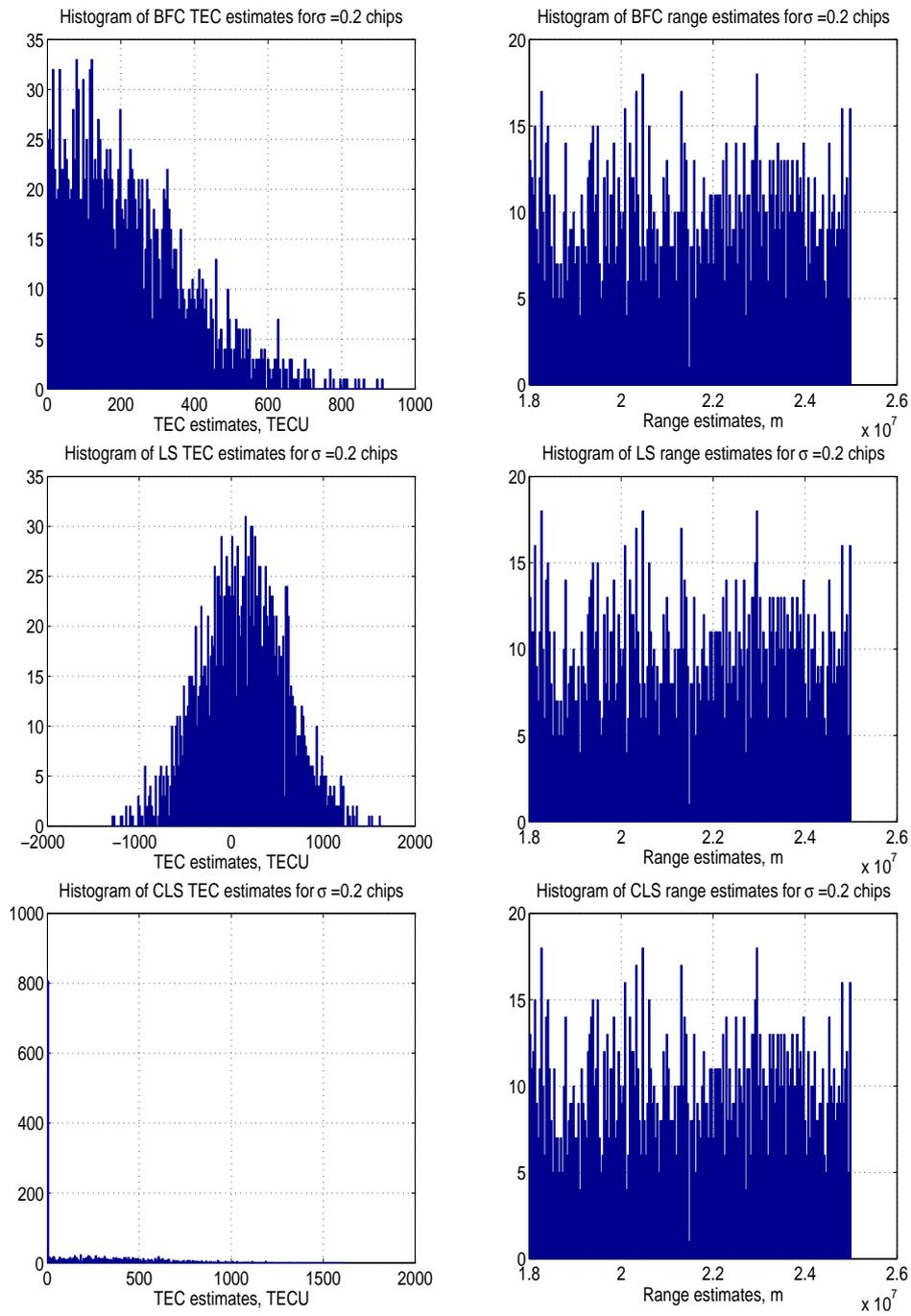
Figure 4: Histograms of TEC and range estimates of BFC (top plots), LS (middle plots) and CLS (bottom plots), for E1-E5a frequency combination, zero mean and  $\sigma = 0.2$  chips.
