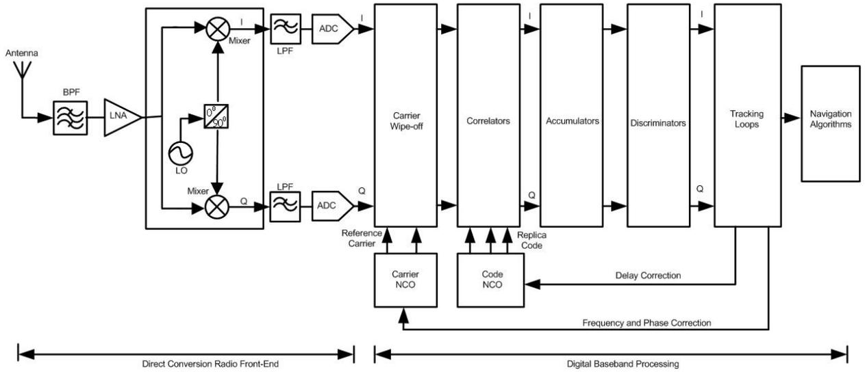
Fig. 1 Block-diagram of a GNSS direct-conversion receiver
