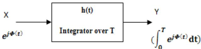
Fig. 2 Equivalent model of phase noise effect
