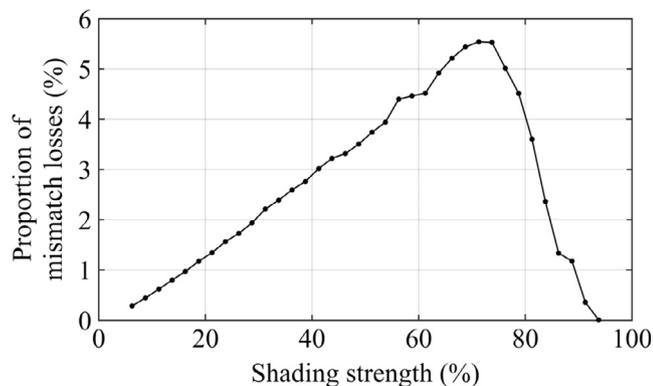
Fig. 7. Proportion of total mismatch losses caused by irradiance transitions with different SSs.
