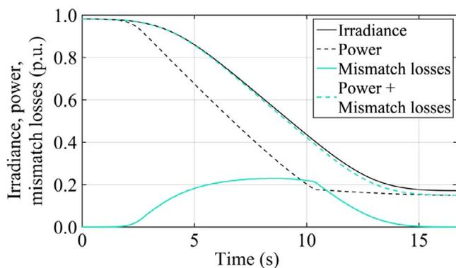
**Fig. 2.** Average irradiance, output power and mismatch losses for the 6 × 28 PV array layout with the SP configuration during partial shading caused by the movement of a shadow edge over the array. Irradiance is with respect to 1000 W/m<sup>2</sup> and power and mismatch losses to the nominal power of the array.
