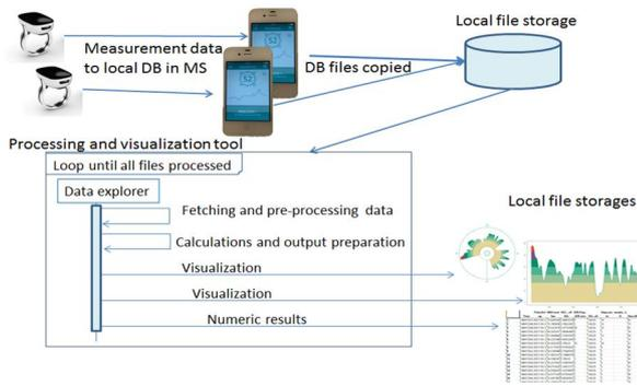
Fig. 1 Process of EDA data processing and visualization.
