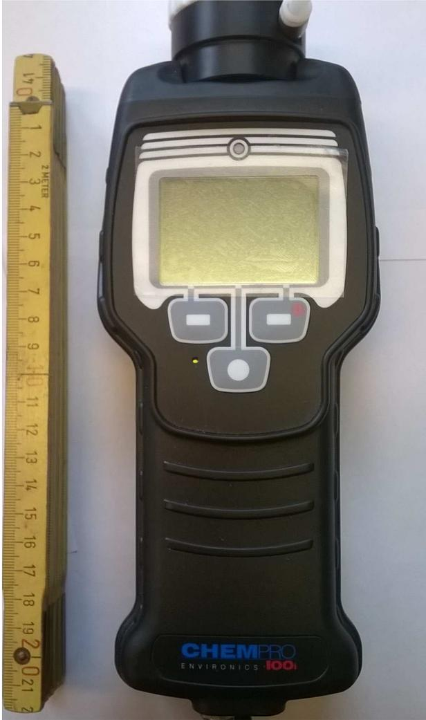
Fig. 1: ChemPro100i handheld chemical detector from Environics with ruler showing values in centimetres.
