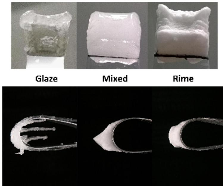
Figure 2. Different ice types formed in the icing wind tunnel. Glaze ice, rime ice and mixture of them (mixed ice) on steel plates and aerodynamic profiles. Modified from (Ref. 1).
