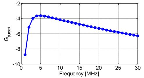
Fig. 2. Simulated link power efficiency ( $G_{p,\text{max}}$ )
