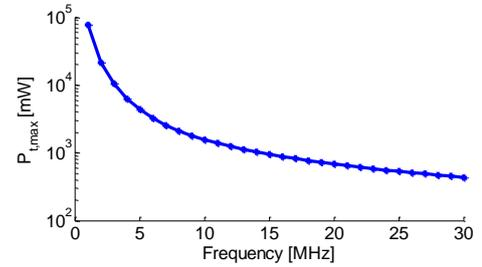
Fig. 3. Simulated maximum SAR-complaint transmission power ( $P_{t,\text{max}}$ ).
