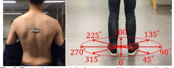
Fig. 2. Tag under test attached to a test subject's upper back during the measurements.
