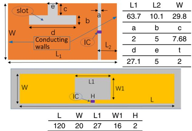
Fig. 1. Structural diagrams of PT (top) and DT (bottom). Dimensional parameters are given in millimeters.
