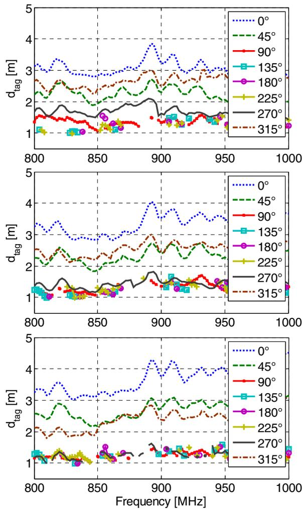
Fig. 3.  $d_{tag}$  of DT worn directly on body (top) and at 5 mm (center) and 10 mm separations (bottom).
