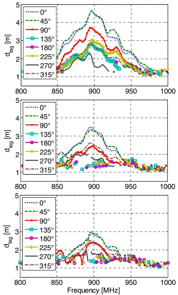
Fig. 4.  $d_{tag}$  of PT worn directly on body (top) and at 5 mm (center) and 10 mm separations (bottom).
