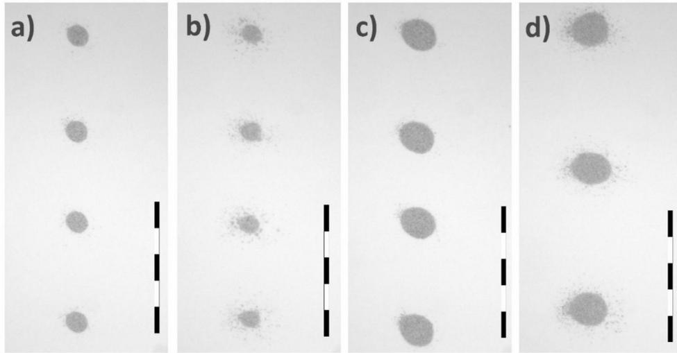
**Figure 3:** Confirmation runs for Nozzle2 with target widths of 7.5µm (a and b) and 12.5µm (c and d). The print height in a) and c) is 50 µm and in b) and d) 70 µm. Lower print height seems to produce more uniform droplets. Scale bar is 50 µm.
