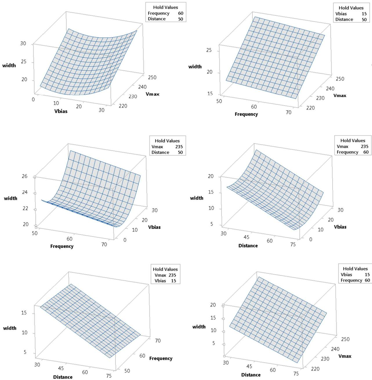
**Figure 2:** Response surface plots for different factor combinations. The width and distance ( $h$ ) are in micrometers, the  $V_{max}$  and  $V_{bias}$  in Volts, and frequency ( $f$ ) in Hertz.
