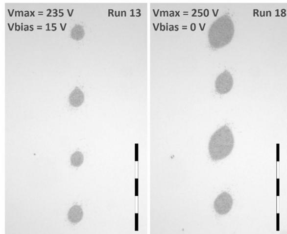
**Figure 3:** Confirmation runs printed with and without  $V_{bias}$ . Printing speed varied between runs. Scale bar is  $50 \mu\text{m}$ .
