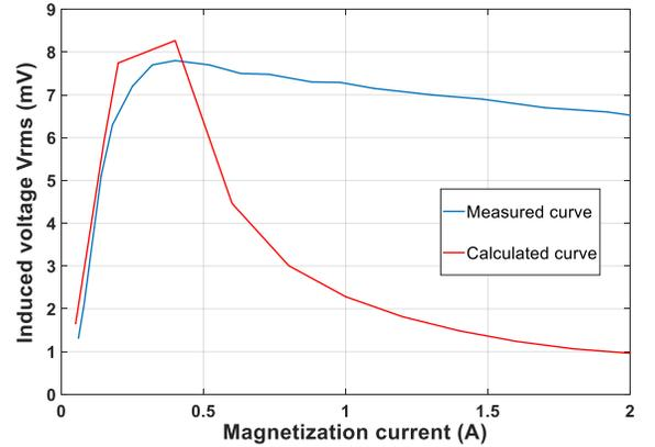
Fig. 3. Induced voltage in the pickup coil.
