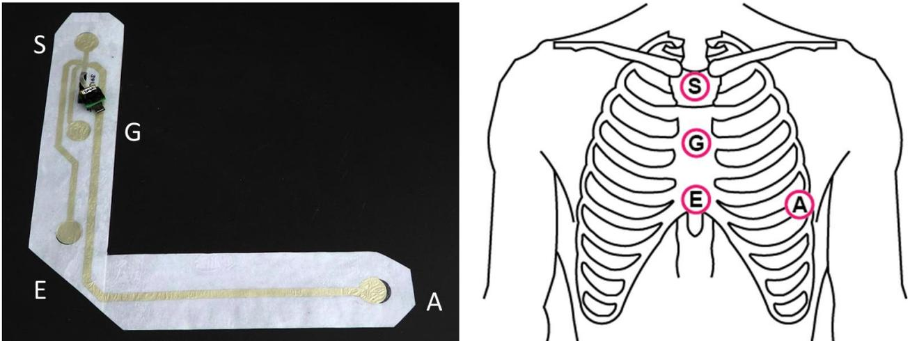
Figure 2. The monitoring system and printed electrode placement.
