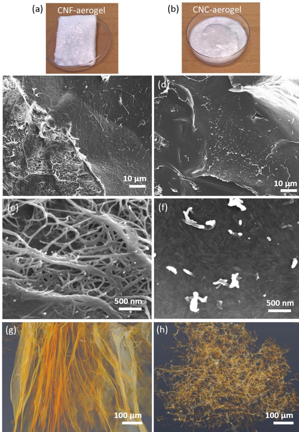
Fig. 1. Photographs of (a) CNF and (b) CNC aerogels. Scanning electron microscope (SEM) images of the (c, e) CNF and (d, f) CNC aerogels surfaces.  $\mu$ CT (X-ray micro-computed tomography) images of (g) CNF and (h) CNC aerogels.
