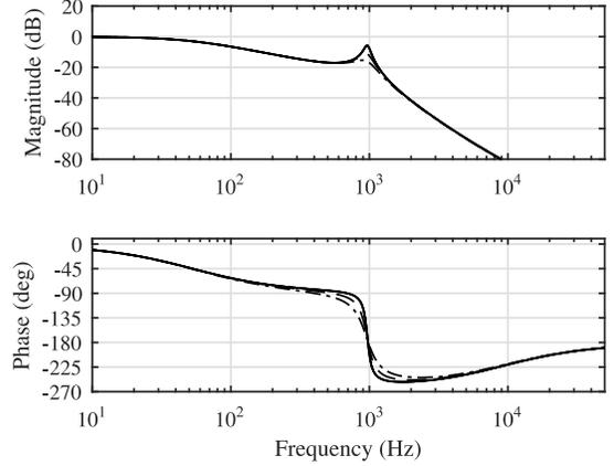
Fig. 6. Estimated frequency response of the closed-loop control-to-input voltage transfer function under I control in different operation regions (CCR: solid line, CPR: dashed line, CVR: dash-dotted line).
