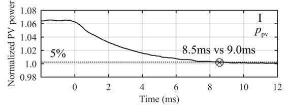
Fig. 13. The measured power-transients induced by a step change in PV voltage in CCR under I control.
