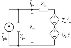
Fig. 3. The dynamic representation of the PV-generator-converter interface.
