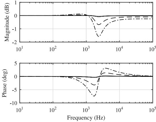
Fig. 5. Predicted PV-generator effect on the closed-loop transfer functions of an input-voltage-feedback-controlled boost power-stage converter (i.e.,  $1/(1+Z_{in-c}/r_{pv})$ ), where the crossover frequency of the input-voltage feedback loop is placed higher than the resonant frequency (i.e., 1 kHz vs. 3 kHz).
