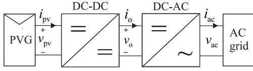
Fig. 2. A grid-connected two-stage PV system.
