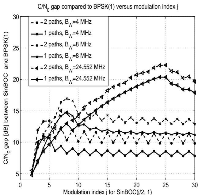
Fig. 3. Minimum  $C/N_0$  gap between  $\text{SinBOC}(j/2, 1)$  modulation and  $\text{BPSK}(1)$  for two-path channel.
