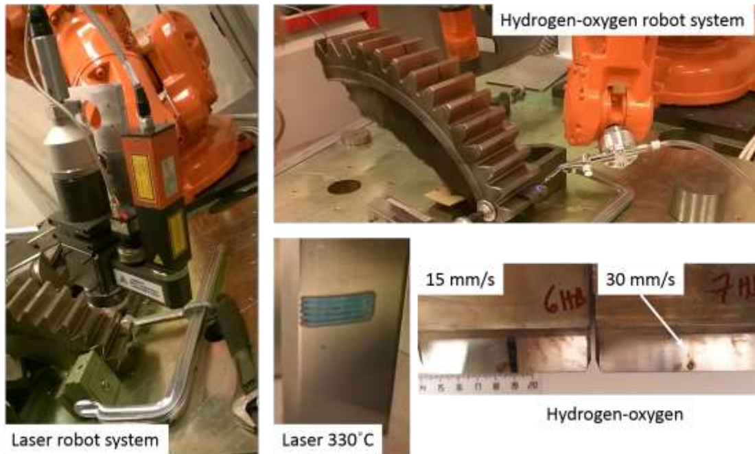
Figure 1. Robotic assembled laser system and hydrogen-oxygen flame burner system with examples of produced tempered marks with 330 °C laser and production speeds of 15 mm/s and 30 mm/s with the hydrogen-oxygen burner.
