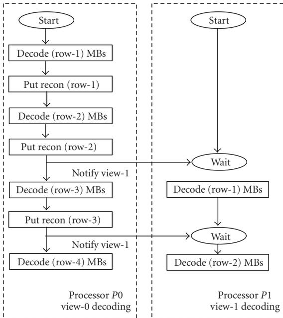
FIGURE 9: Sample parallel decoding process for two views.
