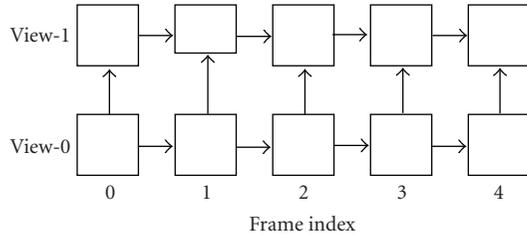
FIGURE 7: Sample prediction structure for two views.
