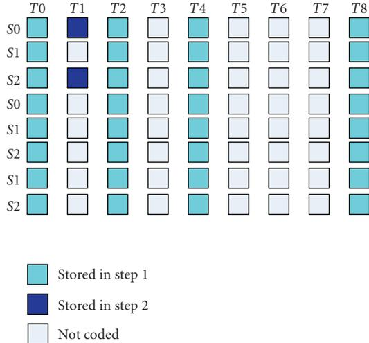
FIGURE 6: DPB status for time-first coding.
