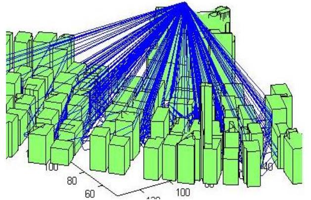
Fig. 1. 3D ray tracing in macro cellular environment.
