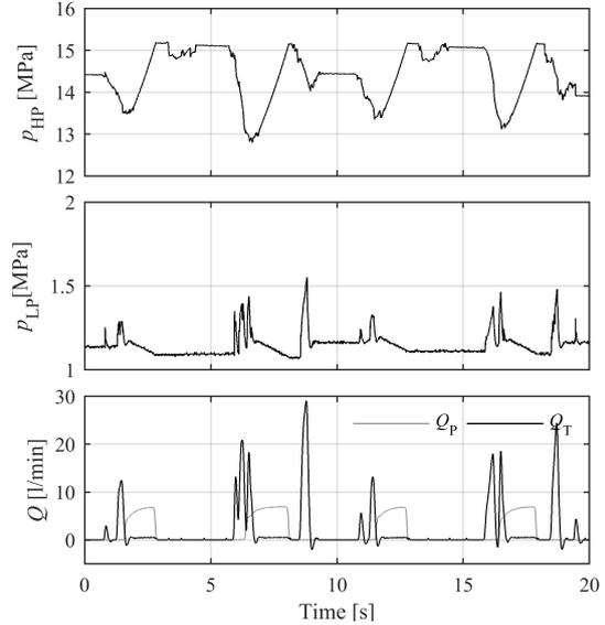
Figure 4: Measured pressures and flow rates
