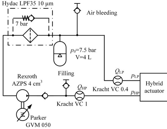
Figure 3: Hydraulic circuit diagram of the test setup. The hybrid actuator includes a HP accumulator.
