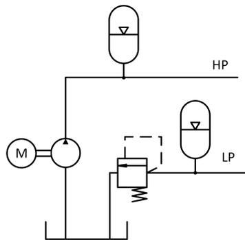
Figure 1: Pressurized tank concept with pressure relief valve in LP line
