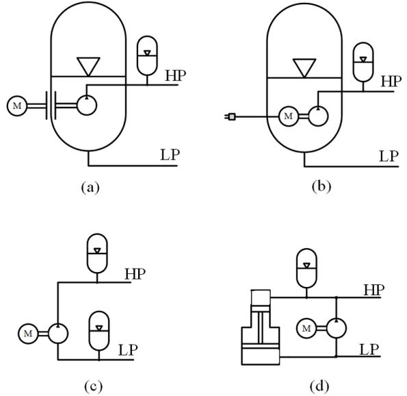
Figure 2: Four different implementation alternatives of pressurized tank without a pressure relief valve in LP line
