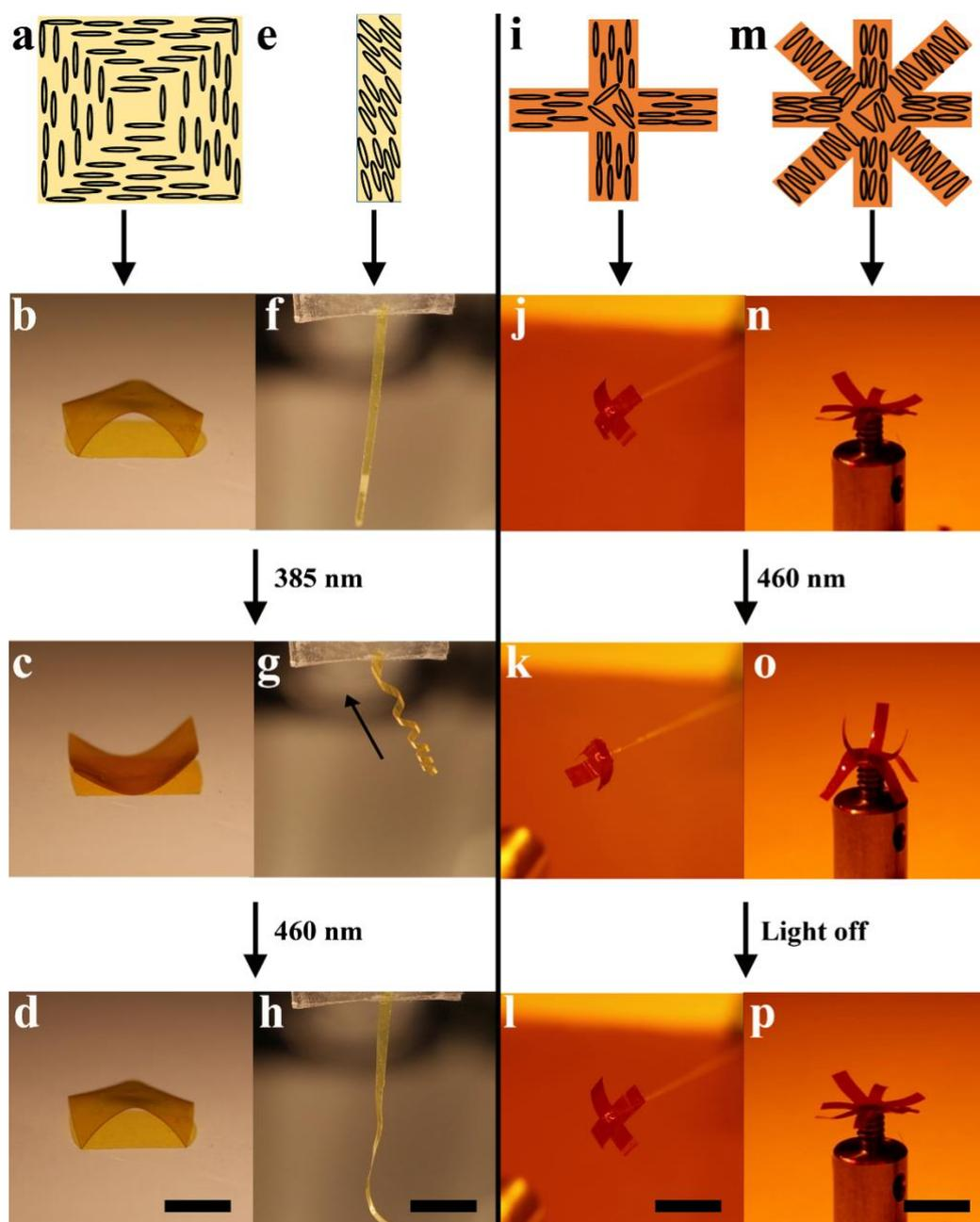
**Figure 4.** Molecular orientation and actuation via photochemical mechanism of (a-d) a film with +1 topological defect; (e-h) a film stripe with modified director angles from one end to the other. Photothermally actuated 4-armed gripper (i-l), and 8-legged "insect" structure (m-p). All scale bars correspond to 6 mm.
