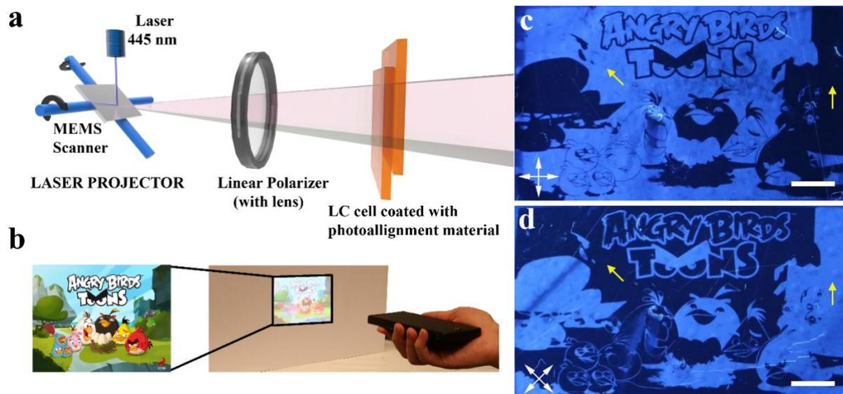
**Figure 1.** (a) Working principle of the photoalignment set-up with the single-mirror MEMS laser projector. (b) Projection of a coloured image by the miniature laser projector. (c) and (d) Polarized microscope images of photopatterned samples. Crossed double-headed arrows represent the polarizer and analyser directions, yellow arrows indicate the local LC alignment orientation. Scale bars: 3 mm. Image in (b) used with permission from Rovio Entertainment Ltd.
