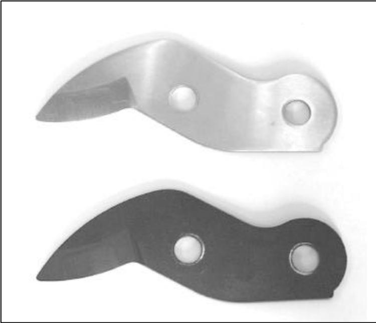
*Figure 15. The chromium-coated steel (upper) and PTFE-coated (lower) lopper blade. Excluding the coating material, the blades are identical.*
