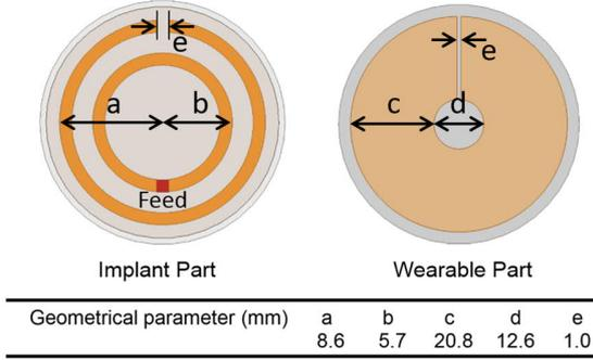
Fig. 1. Antenna system with its geometrical dimensions.
