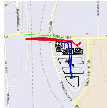
Fig. 1. Example test track with corresponding location references (green), location estimates (blue), and locations provided by GPS (red).
