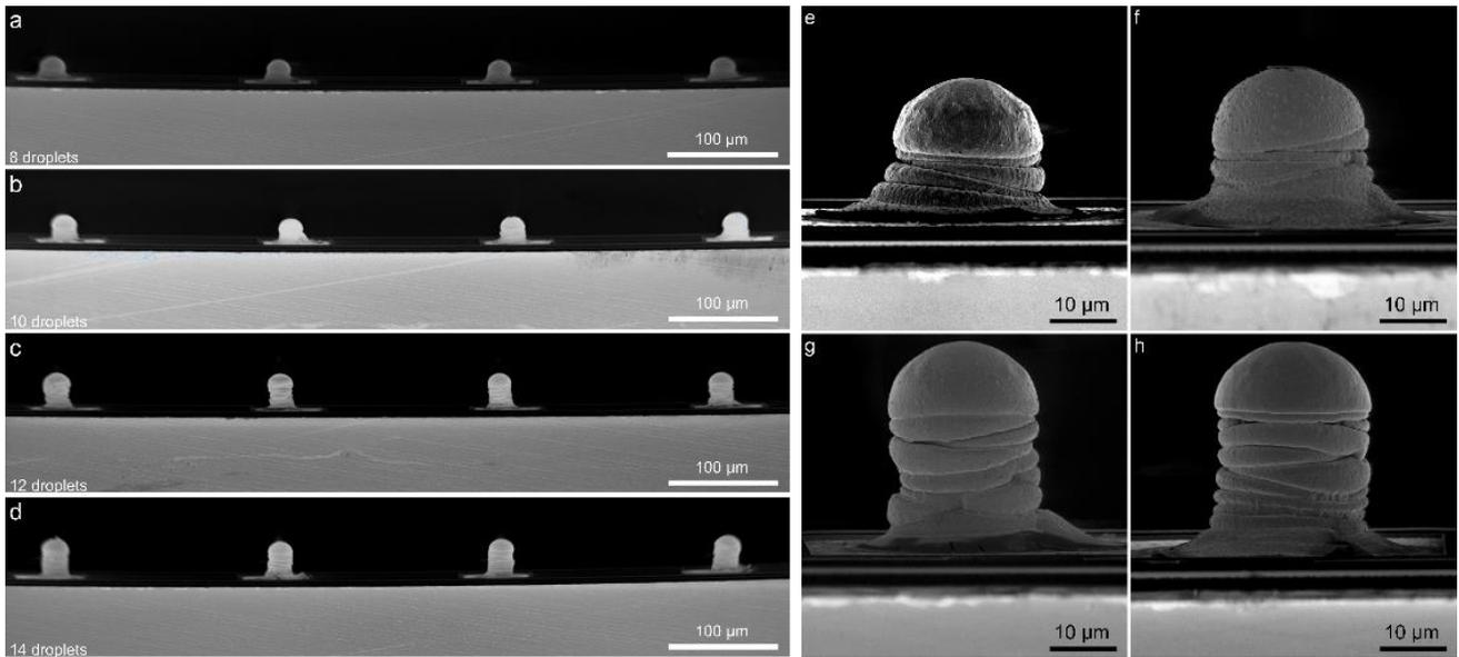
**Figure 7.** SEM images of printed silver pillars on adjacent chips pads (left) with a) 8 droplets ( $20.9 \pm 0.0 \mu\text{m}$ ), b) 10 droplets ( $25.9 \pm 0.8 \mu\text{m}$ ), c) 12 droplets ( $33.3 \pm 1.3 \mu\text{m}$ ), d) 14 droplets ( $35.9 \pm 1.1 \mu\text{m}$ ), and the magnified single pillar (right) of e) 8 droplets ( $22.4 \mu\text{m}$ ), f) 10 droplets ( $24.7 \mu\text{m}$ ), g) 12 droplets ( $31.8 \mu\text{m}$ ), h) 14 droplets ( $33.0 \mu\text{m}$ ).
