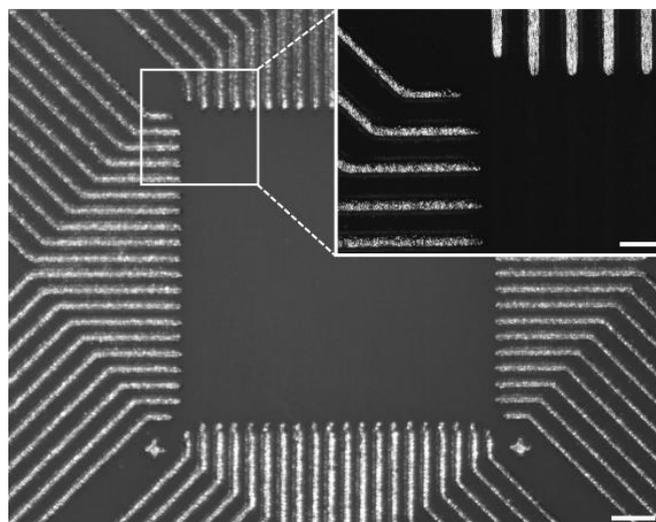
Figure 11. Microscopic image detailing the reduced line lengths of the corner PCB paths (scale bar length =  $500 \mu\text{m}$ ;  $200 \mu\text{m}$  for inset).
