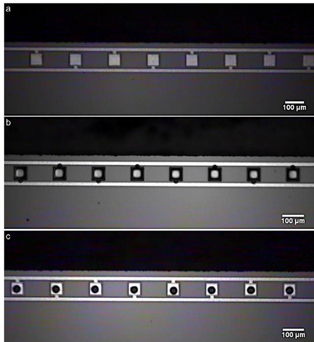
**Figure 4.** Magnified images of the bare die edge with (a) Al pads before printing, (b) printed droplets on the Al pads with no surface treatment and (c) printed droplets on the Al pads with chemical surface treatment.
