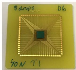
**Figure 5.** Photograph of a bumped test chip bonded to the PCB substrate using flip-chip bonding.
