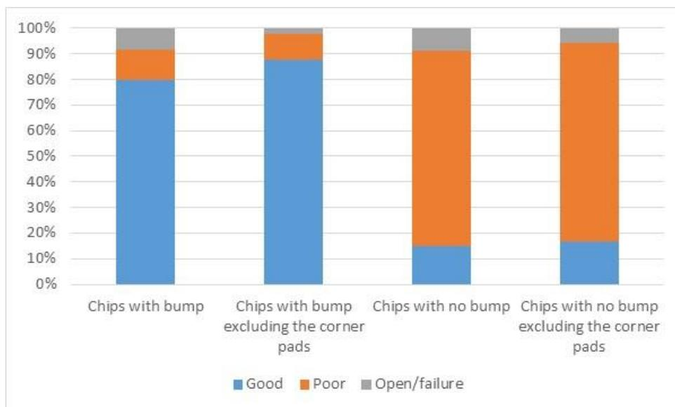
Figure 10. Proportion of I/O connection performance [1] good ( $<5 \Omega$ /pair;  $2.5 \Omega$ /bump + trace), 2) poor ( $5-60 \Omega$ ) and 3) Failure/open circuit ( $>60 \Omega$ )] for bonded samples with or without the printed bumps.
