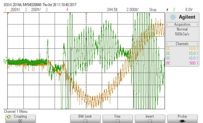
Fig. 5. Voltage (orange) and current (green) when turning on the grid emulation in unstable case. 1.7 mH simulated inductance
