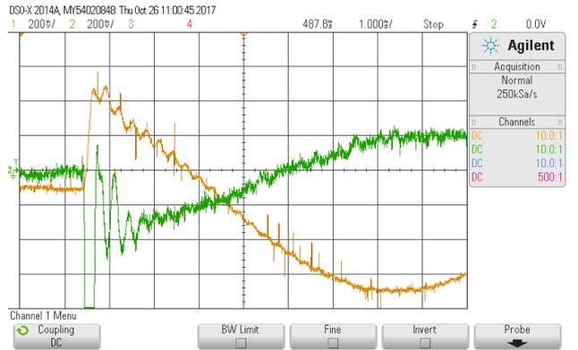
Fig. 4. Voltage (orange) and current (green) when turning on the grid emulation in a stable case. 1.5 mH simulated inductance
