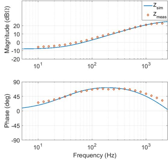
Fig. 3. Measured impedance from the PHIL-test bench (red) and the impedance simulated with the transfer function approximation G (blue).
