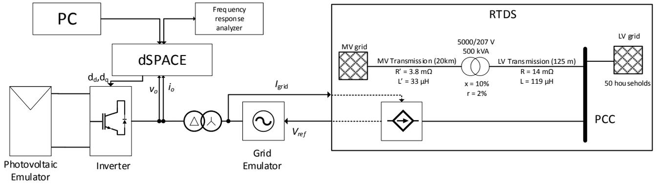
Fig. 1 Layout of the test bench
