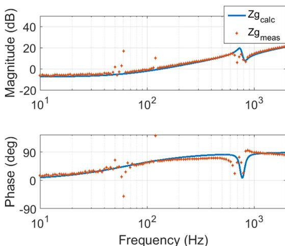
Fig. 6. Measured (red) and calculated (blue) impedances at the hardware side when a resonant frequency in impedance is modeled at 800 Hz
