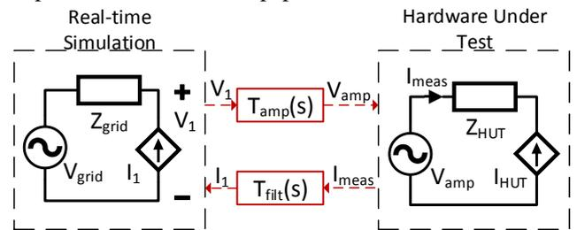
Fig. 2. Control diagram of the PHIL grid emulation with ITM interface algorithm
