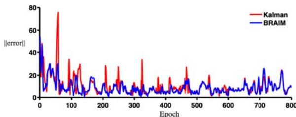
**Fig.6. Errors of Kalman filtered position estimate versus the error given by the BRAIM method on a real GPS data vehicular test.**
