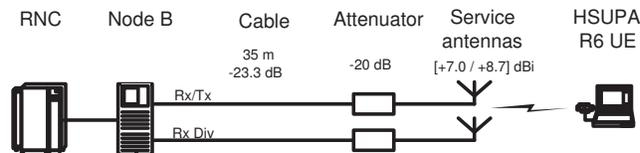
Fig. 1. System block diagram and antenna configuration.
