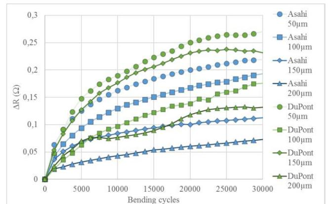
**Figure 9: Estimation of the via bending effect in all eight cases.**
