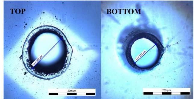
Figure 4: Example of a 100  $\mu\text{m}$  nominal size via.Table 4: Cross section of printed vias (nominal diameters 50, 100, 150 and 200  $\mu\text{m}$ ) using both inks (Asahi and Dupont).
