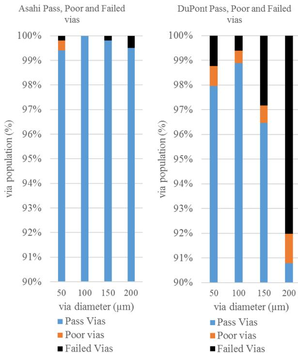
Figure 6: Electrical characterization of via results in eight cases.
