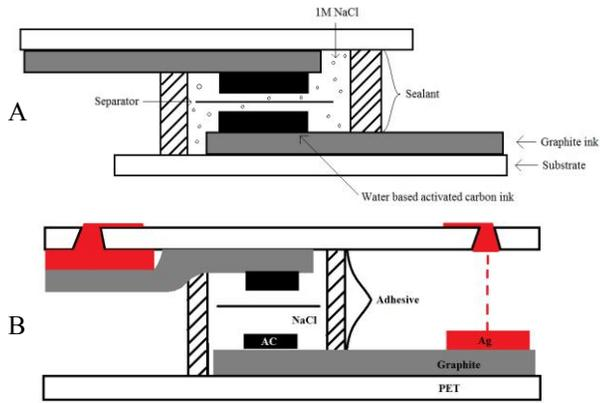
**Figure 11: (A) Supercapacitor reference structure and (B) supercapacitor all sealed structure using vias illustrations.**
