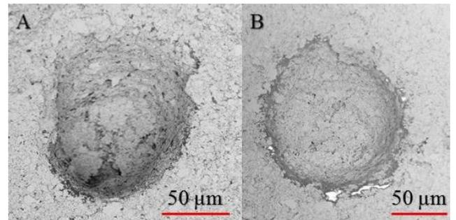
**Figure 10: SEM images of (A) before bent via and (B) after bent via. (100  $\mu\text{m}$  nominal via size)**
