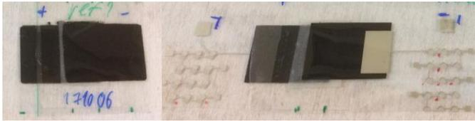
**Figure 12: Reference supercapacitor on the left. Supercapacitor with vias combined structure on the right.**
