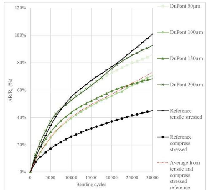
**Figure 8: DuPont samples bending results. Initial resistance ( $R_0$ ) for each case: 50  $\mu\text{m}$ , 16.9  $\Omega$ ; 100  $\mu\text{m}$ , 17.6  $\Omega$ ; 150  $\mu\text{m}$ , 20.0  $\Omega$ ; 200  $\mu\text{m}$ , 12.3  $\Omega$ ; Reference tensile, 9.9  $\Omega$ ; Reference compress 15.5  $\Omega$ .**
