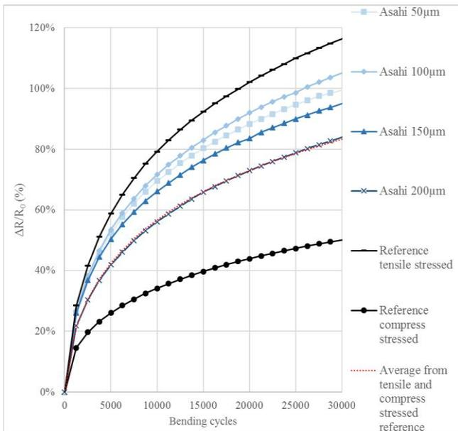
**Figure 7: Asahi samples bending results. Initial resistance ( $R_0$ ) for each case: 50  $\mu\text{m}$ , 13.4  $\Omega$ ; 100  $\mu\text{m}$ , 12.8  $\Omega$ ; 150  $\mu\text{m}$ , 11.9  $\Omega$ ; 200  $\mu\text{m}$ , 11.5  $\Omega$ ; Reference tensile, 10.7  $\Omega$ ; Reference compress 10.5  $\Omega$ .**
