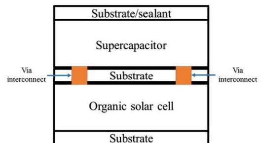
Figure 1: An energy module using screen-printed vias as the interconnection between energy storage and -harvest components.
