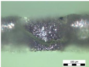
Figure 5: Cross section microscope image of an incomplete screen-printed via with failed connection (150  $\mu\text{m}$  nominal via size).
