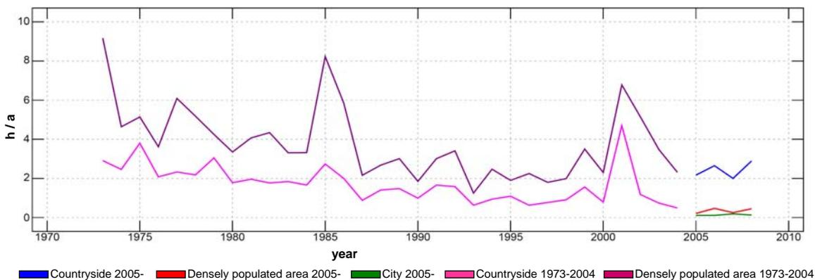
Figure 2.4: The trend of average interruption time caused by faults in the Finnish medium-voltage network from 1973 to 2008 (reclosings are not included). [FEI09]
