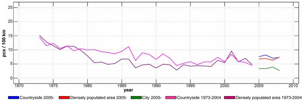
Figure 2.3: The trend of interruption frequency caused by faults in the Finnish medium-voltage network from 1973 to 2008 (reclosings are not included). [FEI09]
