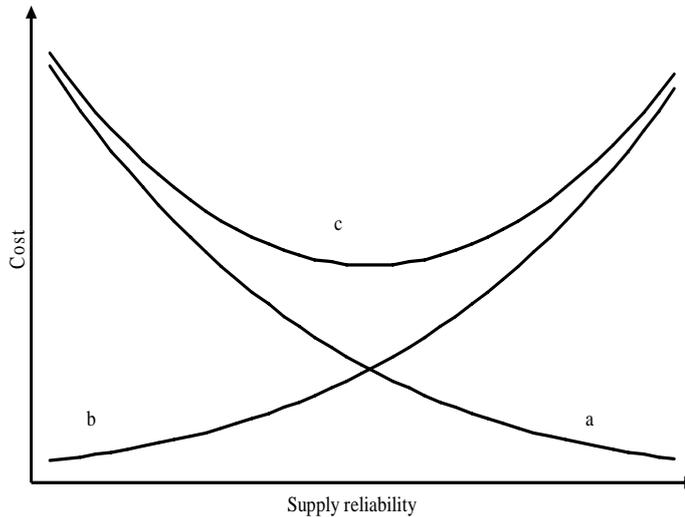
Figure 1.1: Balance between DSO and customer costs.
