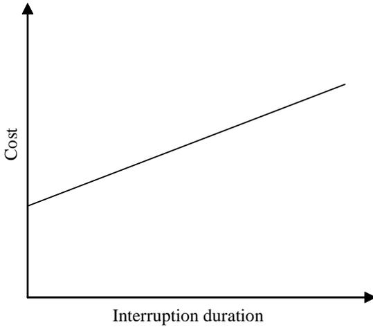
Figure 3.2: Interruption cost functions implied in the combined cost model.
