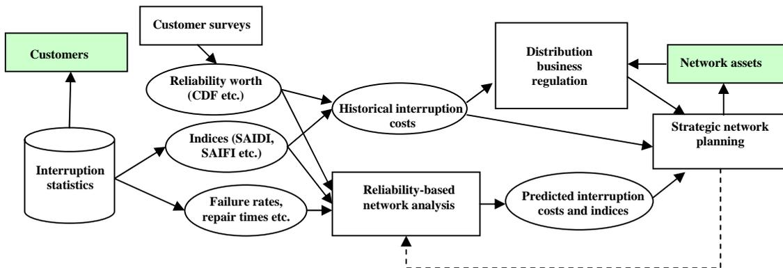
Figure 1.2: Framework of electricity distribution reliability assessment.
