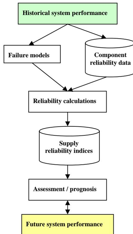
Figure 4.1: Schematic sequence of reliability analysis.
