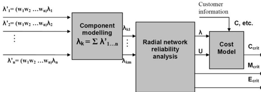
Figure 4.2: Enhanced reliability-based network analysis [PyVe05].
