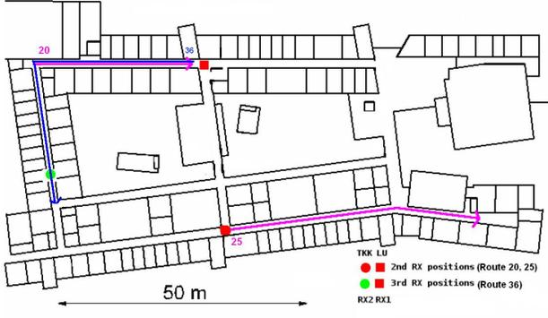
**Fig. 1: Floor plan of the measurement with the TX route (solid line) and the RX position (circle and square)**
