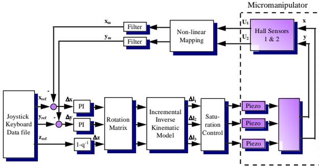
Figure 5: Overview of the controller structure.
