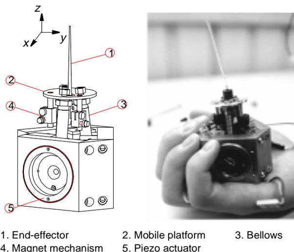
Figure 3: Overview and photograph of the micromanipulator.
