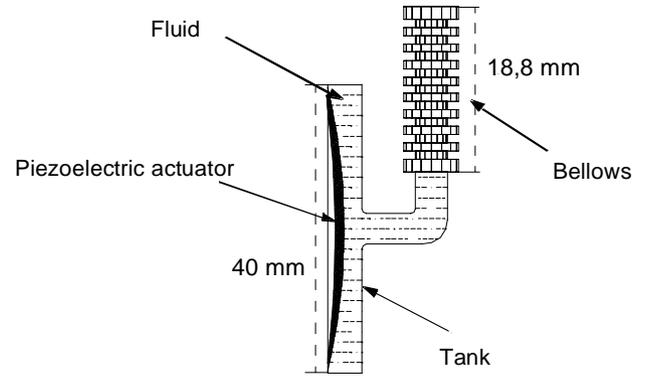
Figure 2: Overview of the actuation system.
