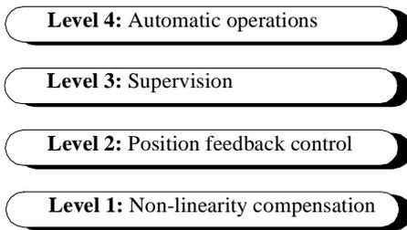
Figure 4: Control levels of the micromanipulator.
