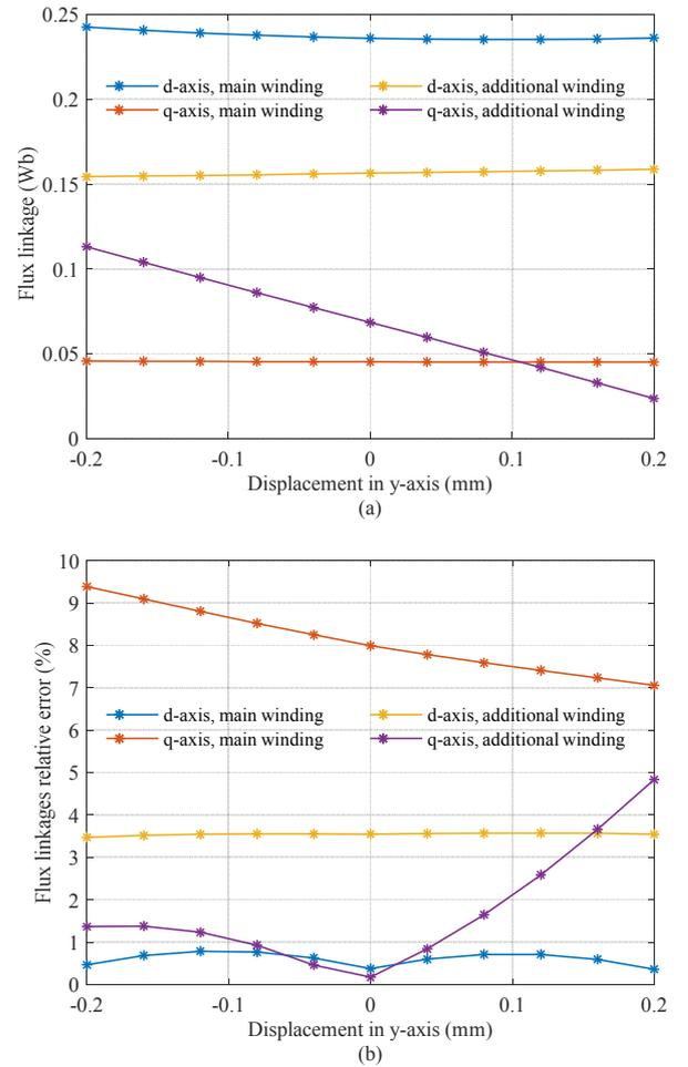
Fig. 6. (a) Flux linkage components, obtained by FE method with respect to the rotor displacement in y-axis; (b) relative error percentage of flux linkages in main and additional windings, calculated from FE method and OIM.
