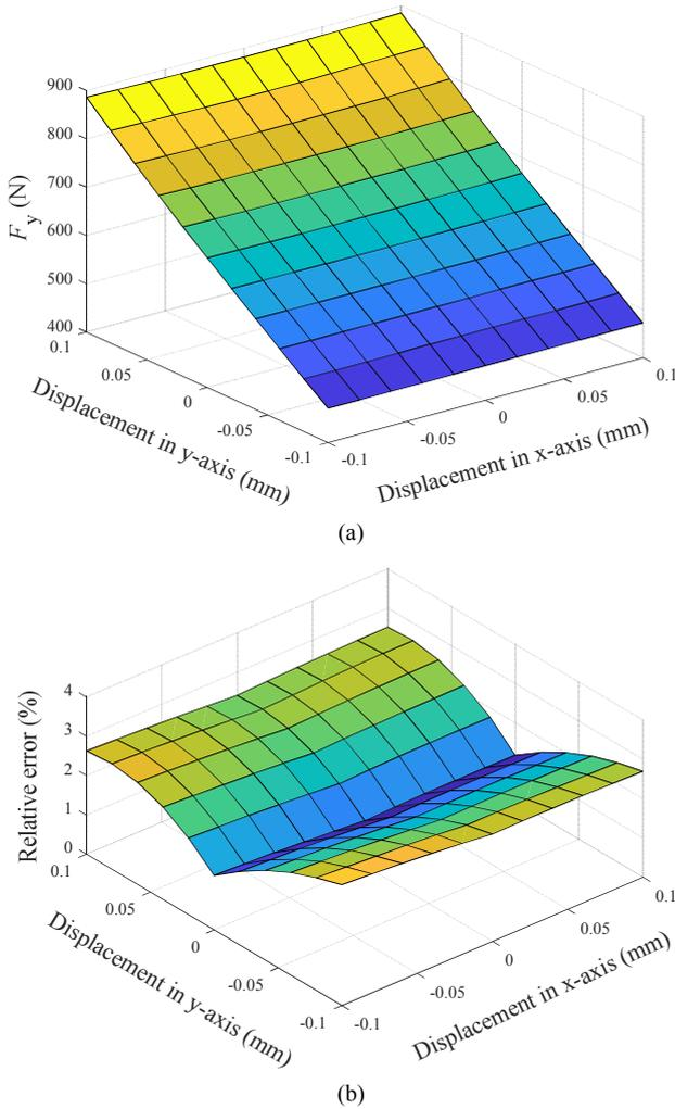
Fig. 7. (a) The electromagnetic force in y direction computed as a function of the displacement of the rotor in x- and y-axes using FE method, (b) the relative error percentage of forces, calculated from FE method and OIM method.
