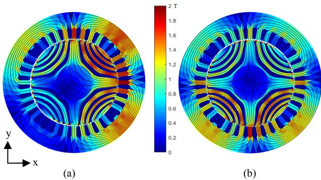
Fig. 3. Magnetic flux density distribution of the motor at rated current in main and additional winding when the rotor is (a) eccentric in positive x-direction, (b) eccentric in negative y-direction.
