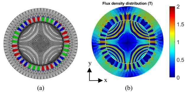
Fig. 1. (a) The first order mesh of the prototype with two windings, the additional winding can be seen in the bottom of the slots, (b) the magnetic flux density of the motor during the rated load and levitation force production state. Unequal flux density distribution between upper and lower parts of the airgap can be noticed.
