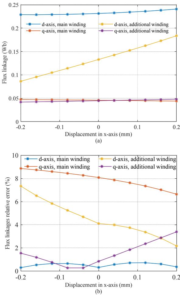
Fig. 5. (a) Flux linkage components, obtained by FE method with respect to the rotor displacement in x-axis; (b) relative error percentage of flux linkages in main and additional windings, calculated from FE method and OIM.
