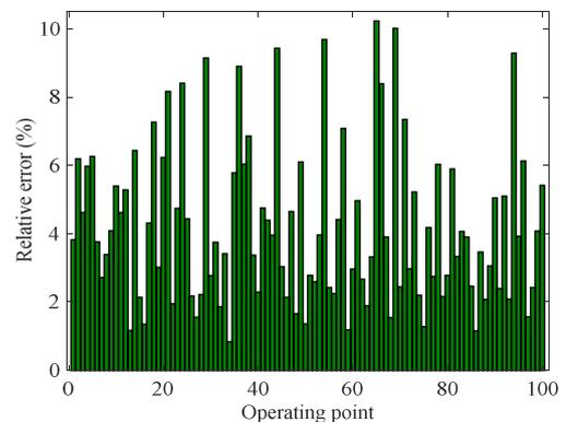
Fig. 4. Percentage of relative error between the nodal values of the magnetic vector potentials obtained by FE method and OIM at different operating points.
