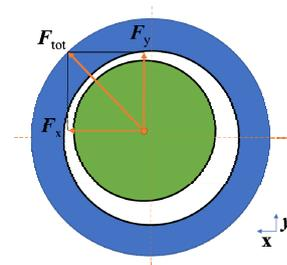
Fig. 2. The rotor center is displaced  $x$  units in the negative x-axis and  $y$  units in positive y-axis from the stator center, as a result the electromagnetic force has been produced towards the shortest airgap.
