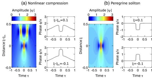
FIG. 2. Detailed view of amplitude and phase dynamics for (a) compression of a higher order  $N = 6$  soliton and (b) a Peregrine soliton. For clarity in the comparison, the distance scale in (a) is  $\xi - \xi_m$  offset relative to the compression point.
