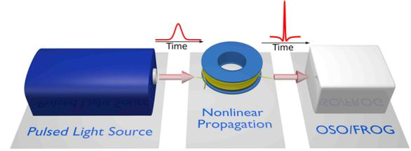
FIG. 3. Schematic experimental setups. The pulsed light source is either a fiber picosecond laser or a spectrally filtered femtosecond OPO. The nonlinear propagation of pulses is achieved in a HNLF or in a standard PMF fiber.
