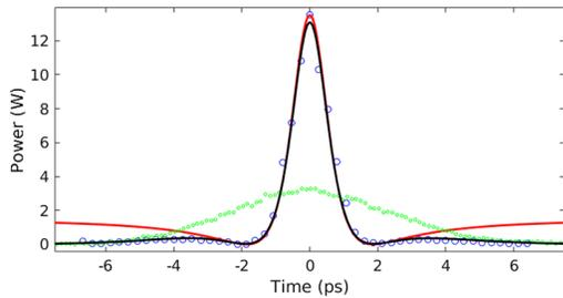
FIG. 4. Experimental and numerical simulations: temporal dynamics of the optical power (setup 1). Input pulse (green points) corresponding to  $N = 1/\epsilon \approx 2.2$ . Output of the 400 m-long PMF (blue circles). Numerical simulations of the NLSE (black line) and theoretical Peregrine soliton (red line).
