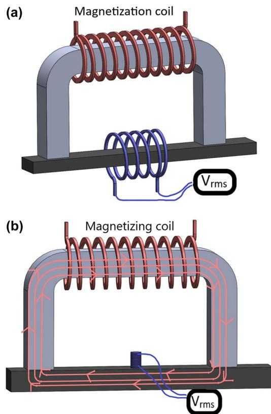
**Fig. 3** **a** Cylindrical coil wrapped around the sample and **b** pickup pancake coil with core and copper winding on the sample surface. Schematic images based on [17]. The formed magnetic fields entering the sample are shown as magnetic flux arrows in (b)
