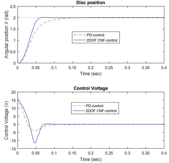
Figure 6. Experimental result: tracking performances of closed-loop systems.
