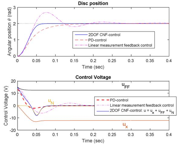
Figure 3. Simulation result: tracking performances of closed-loop systems.
