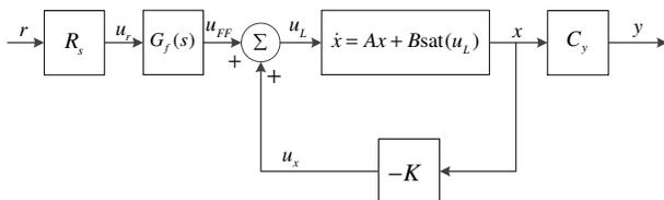
Figure 1. Closed-loop control system with full-state 2DOF controller.
