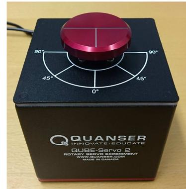
Figure 2. Quanser QUBE-Servo 2 unit with disc attachment.
