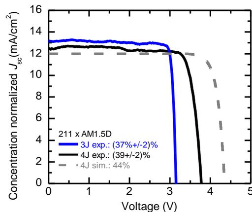
Figure 1. Performance of dilute nitride 3J reference cell, 4J experiment, and performance projection for optimized 4J cell at ~200x.
