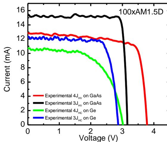
**Figure 1.** IV-characteristics of 3J and 4J cells fabricated on GaAs and Ge substrates by MBE. The 3J cells are fabricated without the 3<sup>rd</sup> junction of the corresponding 4J design. The IV-measurements were biased using continuous 100 suns illumination. The cell size was 1 mm<sup>2</sup>.
