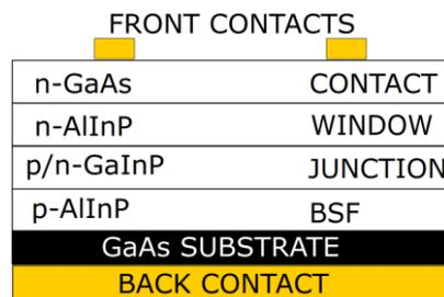
**Figure 1.** Schematic of a solar cell structure under investigation. The lattice-matched structure was grown by molecular beam epitaxy.
