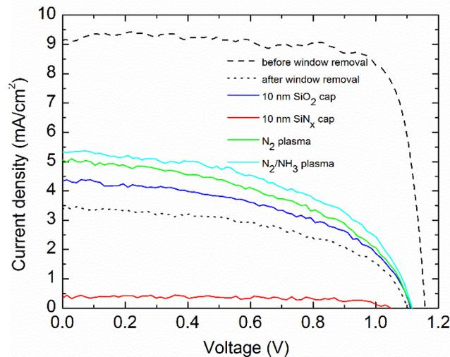
**Figure 2.** Current-voltage performance of 1J GaInP solar cells before and after AlInP window removal (before passivation) and after passivation of the GaInP surface with a SiO<sub>2</sub> cap, a SiN<sub>x</sub> cap, N<sub>2</sub> plasma treatment, and N<sub>2</sub>/NH<sub>3</sub> plasma treatment. Antireflection coatings were not applied.
