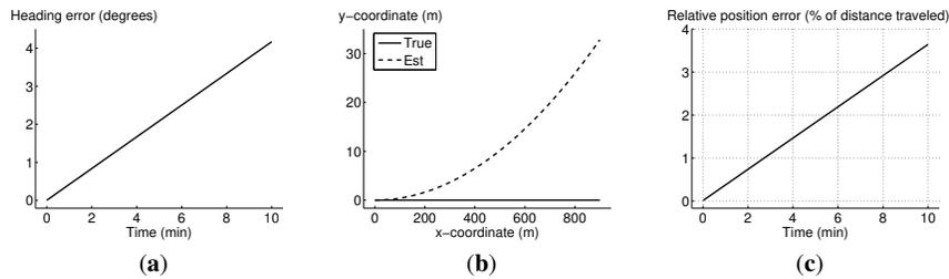
**Fig. 7** Effect of 25°/h gyro bias when the pedestrian is walking with constant speed along the positive  $x$ -axis: (a) heading error; (b) true and estimated coordinates; (c) relative position error
