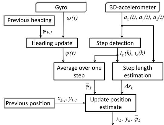
**Fig. 6** Block diagram of the PDR algorithm.
