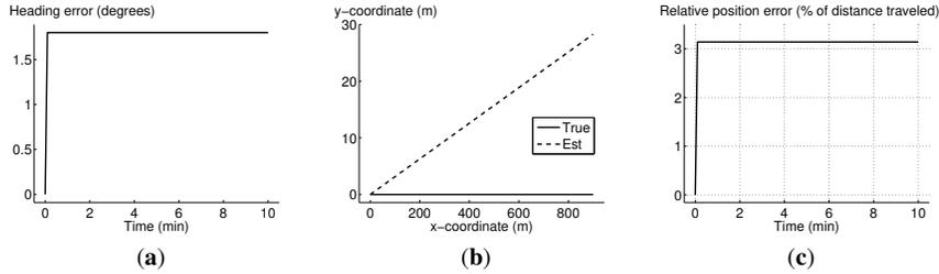
**Fig. 8** Effect of 1% gyro scale factor error when the pedestrian has made a 180 $^{\circ}$  turn from  $-180^{\circ}$  and then walks with constant speed along positive  $x$ -axis: (a) heading error; (b) true and estimated coordinates; (c) relative position error
