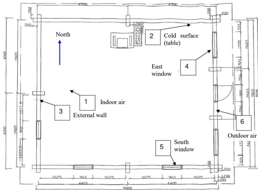
Fig. 2. Location of dataloggers in case building 5.
