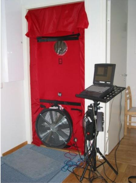
Figure 1. Blower-door system installed on door frames.
