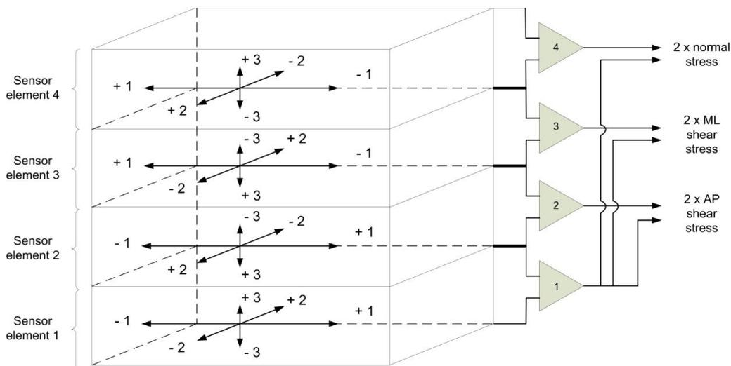
Figure 12. The normal stress (direction 3) and AP (direction 1) and ML (direction 2) shear stresses are obtained as difference signals between the sensor elements.
