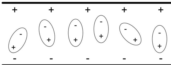
Figure 5. Simplified model structure and typical charge distribution of PVDF material [75].
