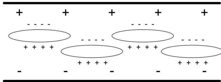
Figure 7. Simplified model structure and typical charge distribution of EMFi [75].
