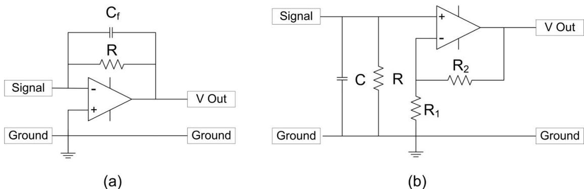
Figure 9. (a) Charge amplifier and (b) non-inverting voltage amplifier.
