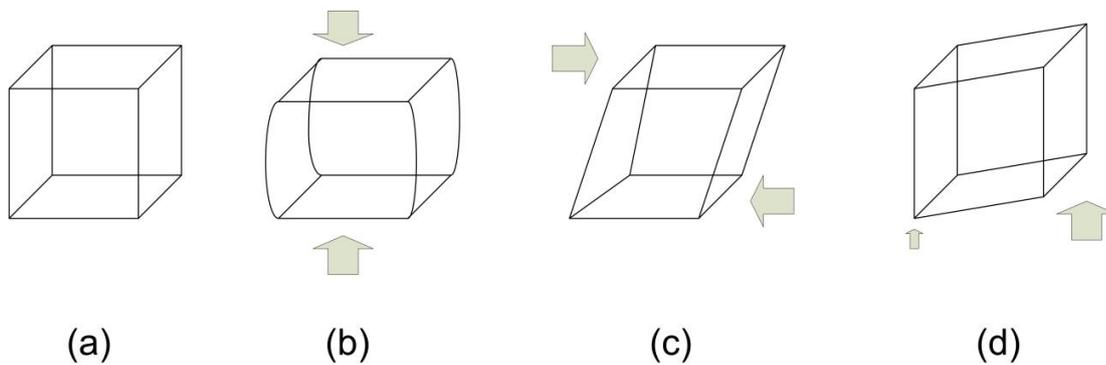
Figure 11. (a) Unloaded cube, (b) the effect of compressive stress, (c) the effect of shear stress and (d) the effect of pinch stress [105].
