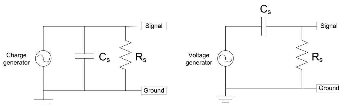
Figure 8. Equivalent circuits of PVDF and EMFi sensors.
