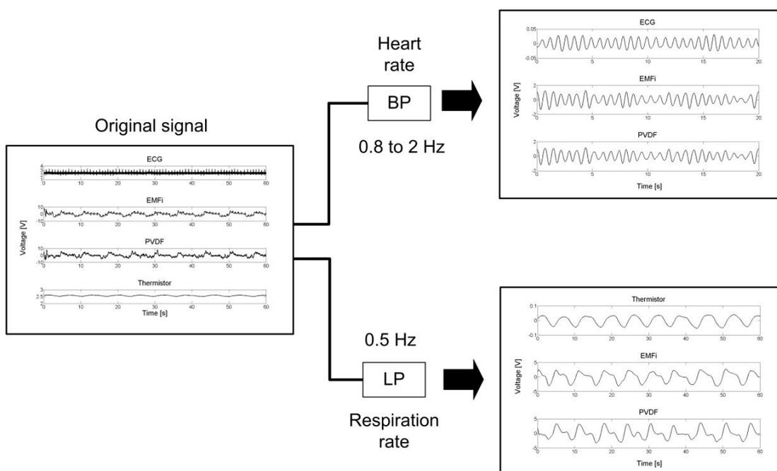
Figure 10. The original signals measured with PVDF and EMFi sensors are filtered to reveal the heart pulsation and respiration components (Butterworth second order bandpass (BP) and lowpass (LP) filters). ECG is used as a reference signal for the heart rate and a nasal thermistor for the respiration.
