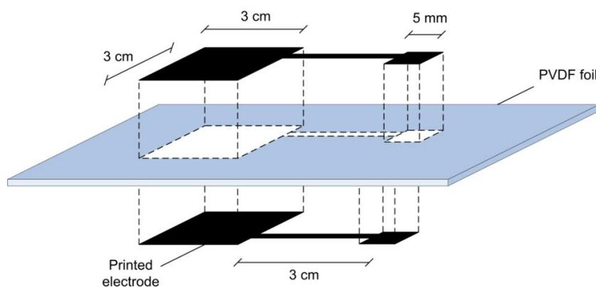
Figure 13. Schematic of the PVDF sensor with printed electrodes.
