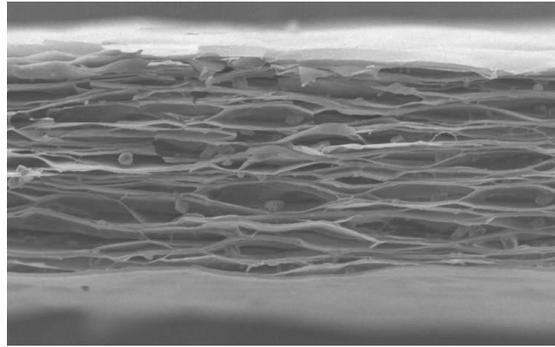
Figure 6. The structure of EMFi material. Photo: courtesy of VTT.
