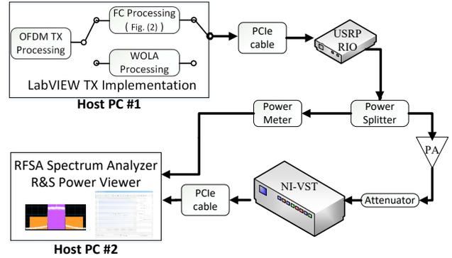
Fig. 1: Block diagram of the considered USRP-based SDR prototype measurement setup.
