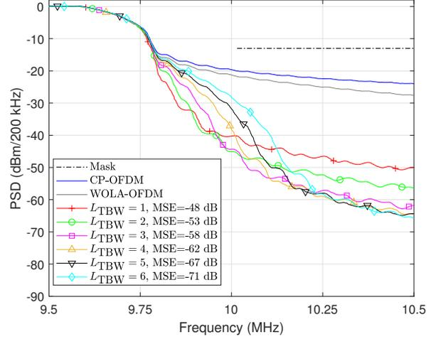
Fig. 3: Example power spectral densities (PSD) close to channel edge for FC-F-OFDM waveforms with different number of transition-band bins for 20 MHz channel with 60 kHz SCS and 27 PRB allocation. Responses for plain CP-OFDM waveform and WOLA-OFDM waveform are shown as a reference.
