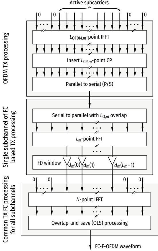
Fig. 2: Block diagram for the FC-F-OFDM transmitter processing of the  $m$ th subband.
