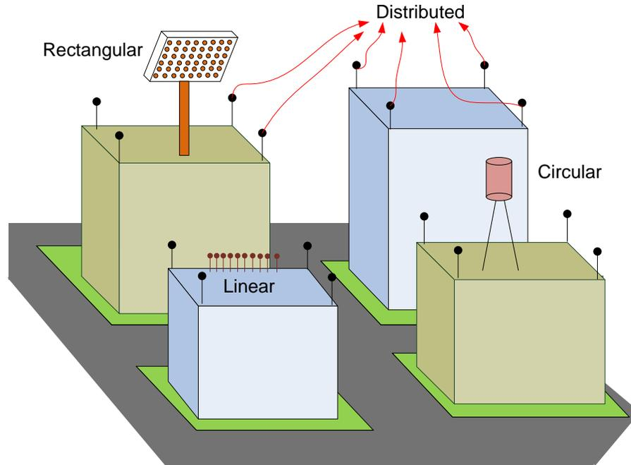
Fig.2. Different antenna configurations for massive MIMO system.
